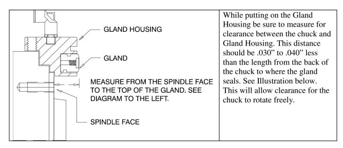
For the FB6-17 the distance from the back of the chuck to where the gland seals is .605 inches. So the distance from the spindle face to the top of the gland should be .565" to .575".
