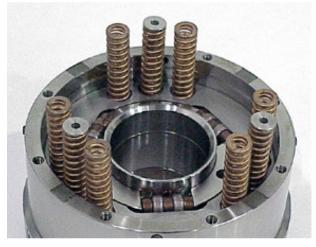
Install the springs into the piston pockets. The springs contain the indicator pin assemblies. (See NOTE and photo on page 9 for a view of indicator pin assembly). They must be installed and aligned with the holes in the faceplate to assure proper chuck operation.
