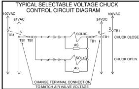
Locate the terminal strip in the electrical cabinet that has the connections for the Chuck Open and Chuck Close solenoids. Locate an area on the electrical cabinet near this terminal strip for the air valves' power cord to enter the cabinet. Drill a pilot hole and use a ½ chassis punch to punch out a hole for the cord grip.
