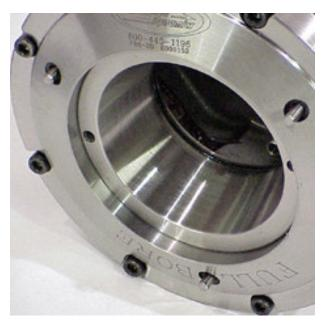
Turn on the air supply to the lathe. The assembled chuck can now be actuated. The pusher will retract when the chuck is in the open, or un-chucked position, and will move forward in the chucked position. Notice the indicator pins moving in and out while the chuck is closed and opened, respectively.
