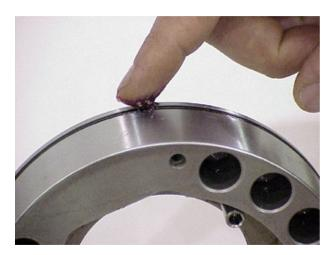
Apply a light coat of grease to both o-rings on the piston and to the I.D. of the body. Gently slide the piston into the chuck body taking care not to wedge the piston in the body.
