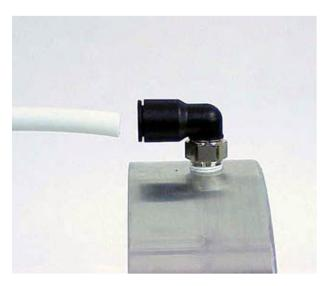
Connect air supply from the valve to the gland housing using the ½" airline supplied with the kit. The port in the gland housing is tapped 3/8 – 18 NPT. Cut off any excess airline and tie up loose or drooping line with wire ties.
